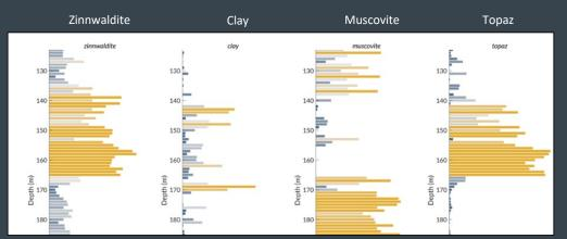
Hyperspectral Imaging 01/2022 by Theiax. Zinnwaldite (ore mineral) easily detectable in a sorting process.
